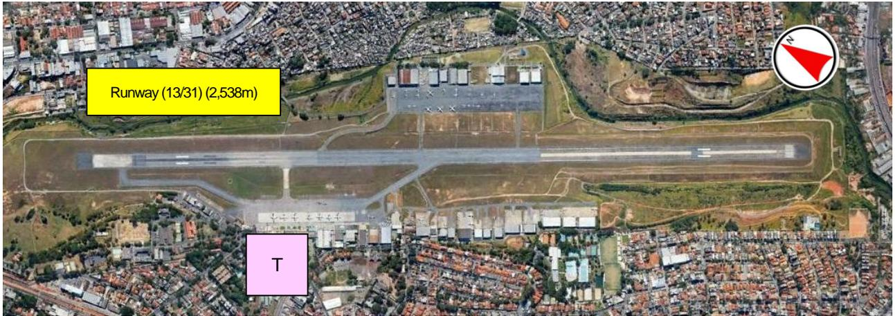
There is a single runway (13/31) with a length of 2,538m. Since 2009, the airport has been equipped with LOC and DME instrument landing systems, which allow the airport to operate under adverse conditions with the same level of operational safety and help reduce the number and time of airport closure by bad weather.
