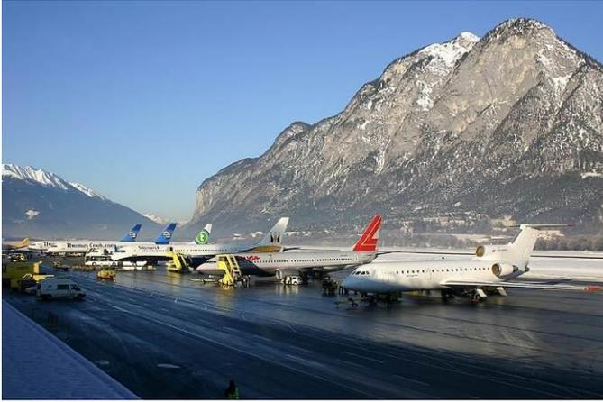
There is one runway of 2,000m (08/26). The terminal is a "shotgun" style, typically using air stairs to deboard/board passengers - no jetways are present. The airport can handle aircraft up to Boeing 767. There are several de-icing trucks, which de-ice the airframe typically right before engines start, or before obtaining clearance to take off.
