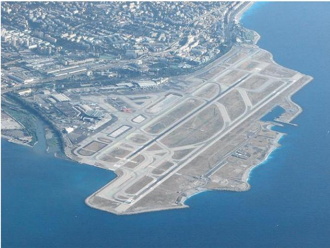
There are one set of close parallel runways; one is the runway (04L/22R) 2,570m and the other is the runway (04R/22L) 2,960m. There are two terminal buildings; Terminal 1 (52,000 m<sup>2</sup>) has 25 gates with a capacity of 4.5 million passengers, Terminal 2 (57,800 m<sup>2</sup>) has 29 gates with a capacity of 8.5 million passengers.
